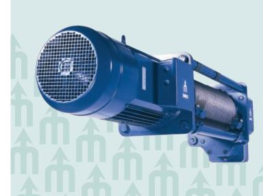
universal, basic configuration that can be placed on a bearing surface, or suspended. The largest hoist model can lift up to 9 metric tons on a single fall of wire rope. Each hoist is available with any of 5 different hoist drums, providing a wide range of lifting heights.
